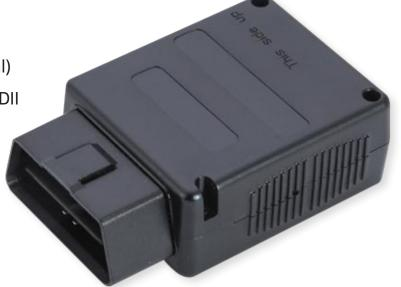
The FM4500 vehicle tracker supports 4G LTE Cat-M1/NB-IoT with fall back to 2G. The FM4500 is a low-cost tracking solution which simply plugs into the OBDII diagnostic port placed in the vehicle, commonly near the driver's knees or below the steering wheel column. Once you plug the FM4500 into the OBDII port of your vehicle, the device starts tracking and monitoring diagnostic information about the vehicle.
